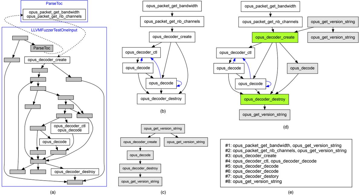
Figure 3: The FuzzGen workflow. FuzzGen starts with a CFG (a) and extracts the corresponding  $A^2DG$  (b) (see (c) for the graph of another module). The two  $A^2DG$  graphs are then merged (d). The merged  $A^2DG$  is then used to create fuzzers based on function orders (e). These graphs are autogenerated by FuzzGen.
