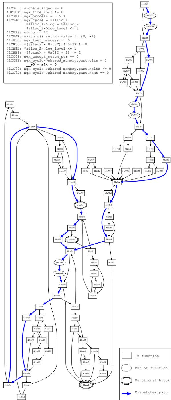
Figure 6: CFG of nginx’s `ngx_signal_handler` and payload for an infinite loop (blue arrow dispatcher blocks, octagons functional blocks) with the entry point at the function start. The top box shows the memory layout initialization for this loop. This graph was created by BOPC.
