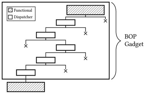
**Figure 2: BOP gadget structure.** The *functional* part consists of a single basic block that executes an SPL statement. Two functional blocks are chained together through a series of dispatcher blocks, without clobbering the execution of the previous functional blocks.
