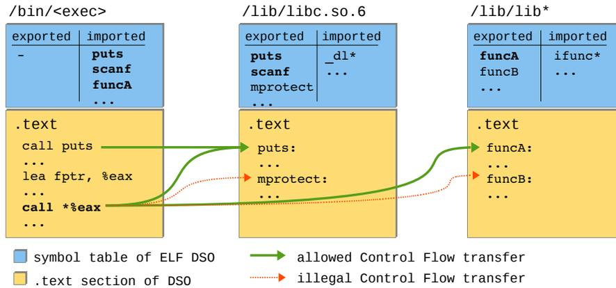
**Figure 2: Call restrictions for an executable and two libraries. Executables and libraries are only allowed to call imported function symbols. Local function calls may only transfer to local function symbols.**
