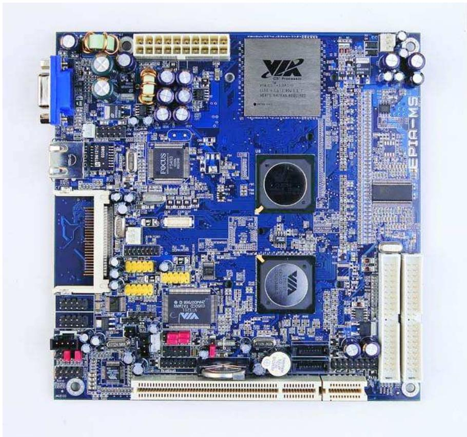
The new kiosk uses a VIA EPIA ML mainboard with a fanless 1 GHz processor. This new mainboard should provide much better hardware stability and the faster processor makes a difference when bigger webpages are displayed.
