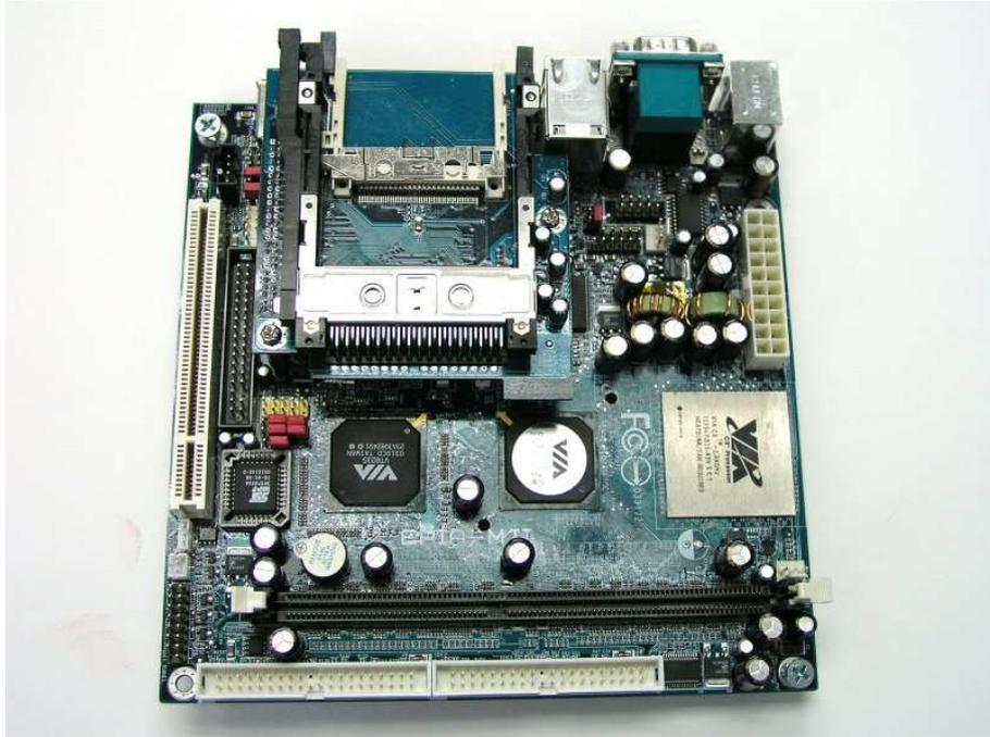
The old kiosk client uses a VIA EPIA MII mainboard with a fanless 600 Mhz processor. This mainboard also has a lot of additional (but in our kiosk unused) features like a CF card slot and a PCMCIA slot.
