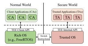
Figure 1: Structure of TrustZone-M based TEE.
