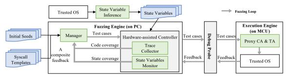
Figure 2: Overview of SYZTRUST. SYZTRUST consists of a fuzzing engine running on a PC, an execution engine running on an MCU, and a debug probe to bridge the fuzzing engine and the execution engine.
