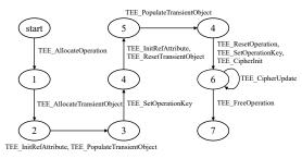
Figure 8: An example of state transition path from the constructed state transition tree in mTower.
