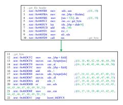
Figure 3: Basic blocks to parse e\_machine.
