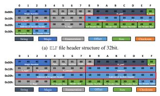
(b) ELF file header structure of 64bit. Figure 1: ELF file header definition.
