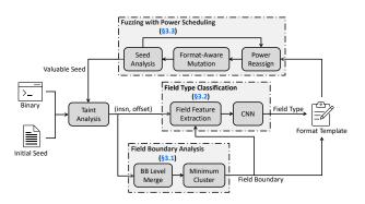
Figure 2: Architecture of AIFORE.
