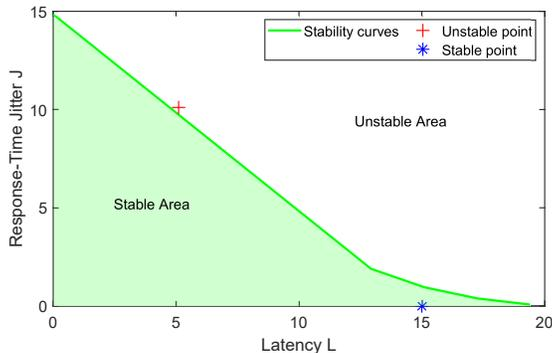
Fig. 5: The stability curve generated by Jitter Margin (the area below the curve is the stable area). The shaded green region is the area in which the plant is guaranteed to be stable. The blue star (latency  $L = 15$  and jitter  $J = 0$ ) shows a stable point and the red plus (latency  $L = 5$  and jitter  $J = 10$ ) shows an unstable point.
