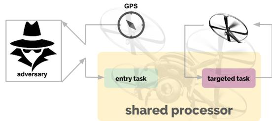
Fig. 1: Illustration of the attack scenario. As a result of intervention (e.g., jamming GPS signals) the entry task consumes less resources and this might lead to instability of the targeted task.
