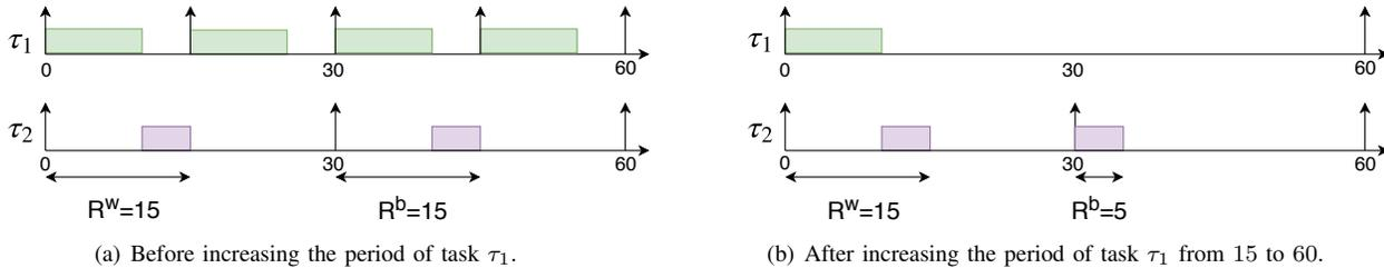
Fig. 4: Schedule of two tasks using a shared platform. The green task has a higher priority and the properties of the tasks are  $\tau_1 = (H, 10, 15)$ ,  $\tau_2 = (L, 5, 30)$ .
