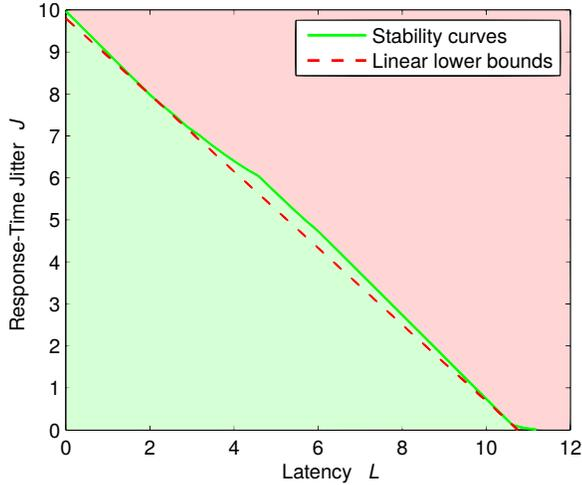
Fig. 3: The stability curve generated by Jitter Margin and the linear lower bound (the area below the curve is the stable area). The curve is generated for a DC servo process with transfer function  $\frac{1000}{s^2+s}$  and a discrete-time Linear-Quadratic-Gaussian (LQG) controller, with a sampling period of 6 ms.
