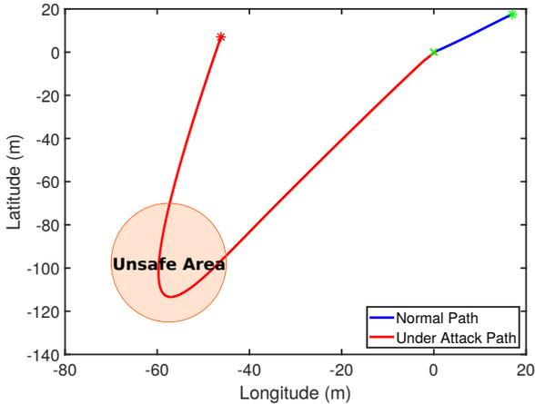
Fig. 12: Two-dimensional position of the quadcopter between time 0s and 4s. The cross and star signs in green show the initial position (0, 0) and desired destination (17, 17) of the quadcopter, respectively. The blue line shows the path of the quadcopter when there is no attack and the red line shows its path when an attack is undergoing. The red star sign at the end of red path shows the position of the quadcopter after 4s, when it is under attack.
